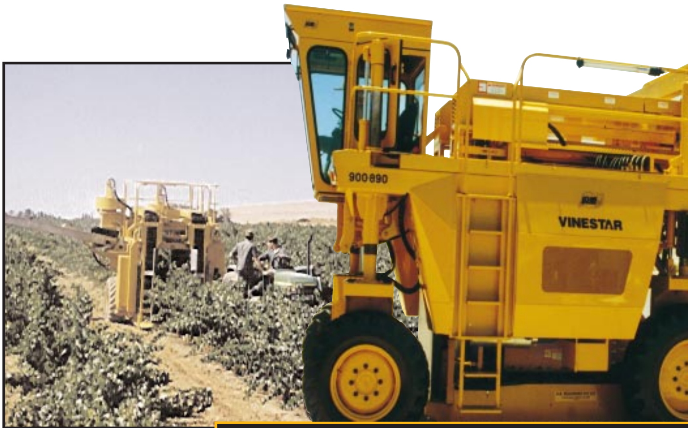
From left: URM Vinestar picking grapes during the 2000 harvest on Walters Family Farm, Malmesbury, South Africa and URM Vinestar self propelled grape harvester.
